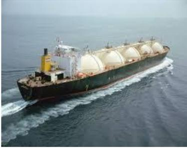
Liquefied Natural Gas is natural gas that has been super-chilled to -260 degrees, turning it into a liquid that is 1/600th the original volume of gas. It is clear, colorless, odorless, and extremely volatile. This gas is compacted so large volumes can be shipped overseas. LNG should not be confused with gasoline or compressed natural gas.
